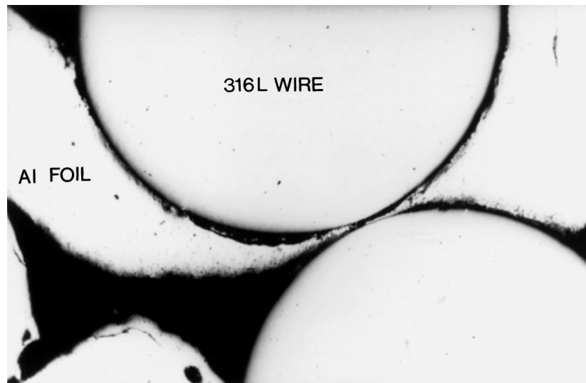
Figure 10 HIPped (F-W-M) 0.5 mm uncoated 316L wires, 0.6 mm Al wires and 0.15 mm Al foil. Al foil is being 'cut' between two 316L wires. Unetched.
