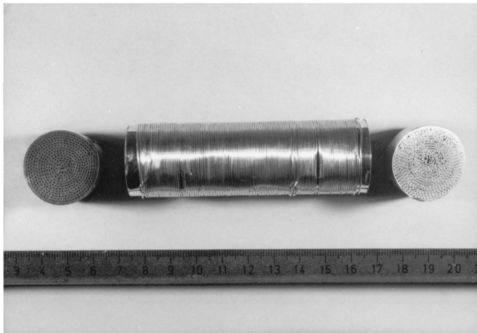
Figure 2 Bundle arrangement (F-W-M). 0.5 mm 316L stainless wires are dark spots in the cross-section and are separated by 0.6 mm aluminium wires (white spots) and 0.15 mm thick aluminium foil.
